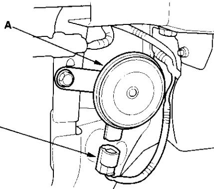
3. Test the horn by connecting battery power to the terminal (A) and grounding to the bracket (B). The horn should sound.
