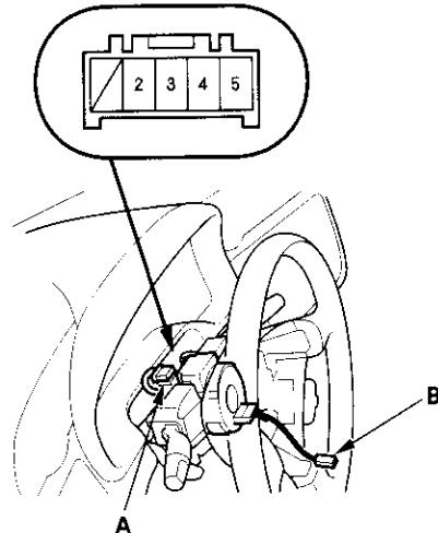
6. Using a jumper wire, connect the horn switch positive 1P connector (B) to ground.
