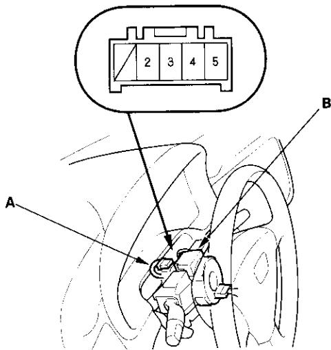
3. Check for continuity between the cable reel No. 2 terminal and body ground with the horn switch pushed. There should be continuity. If there is no continuity, go to step 4.
